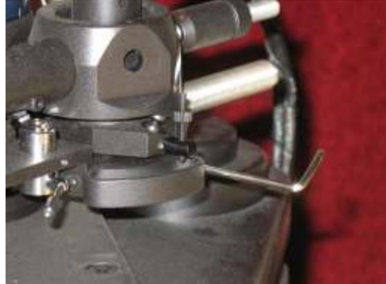
Fig.14 Removing horizontal trough
