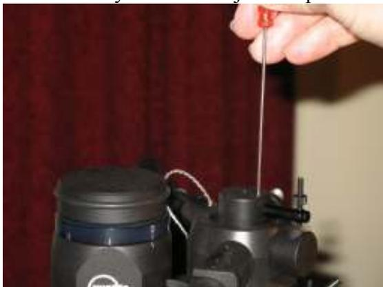
Fig.12. Fixing vertical damping holder
