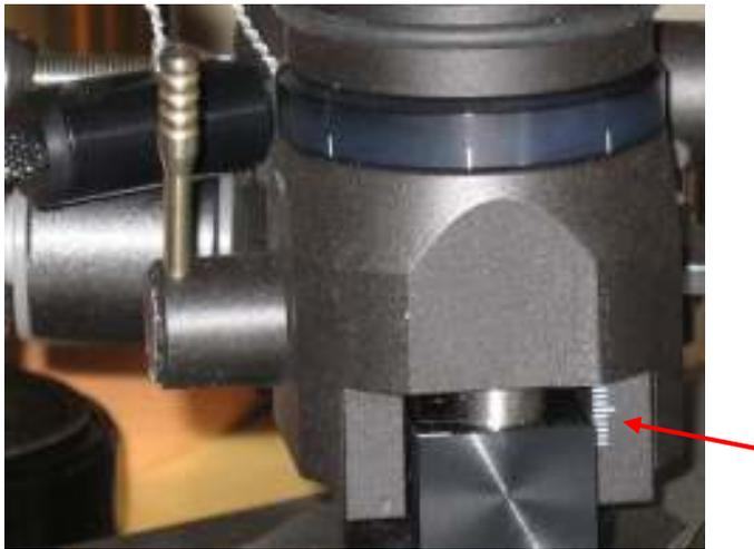
Fig. 10. VTA tower side-rough scale
